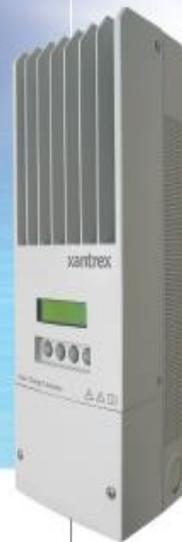
The Xantrex XW Solar Charge Controller is a photovoltaic (PV) charge controller that tracks the electrical maximum power point of a PV array to deliver the maximum available current for charging batteries. When charging, the XW Solar Charge Controller regulates battery voltage and output current based on the amount of energy available from the PV array and state-of-charge of the battery.
