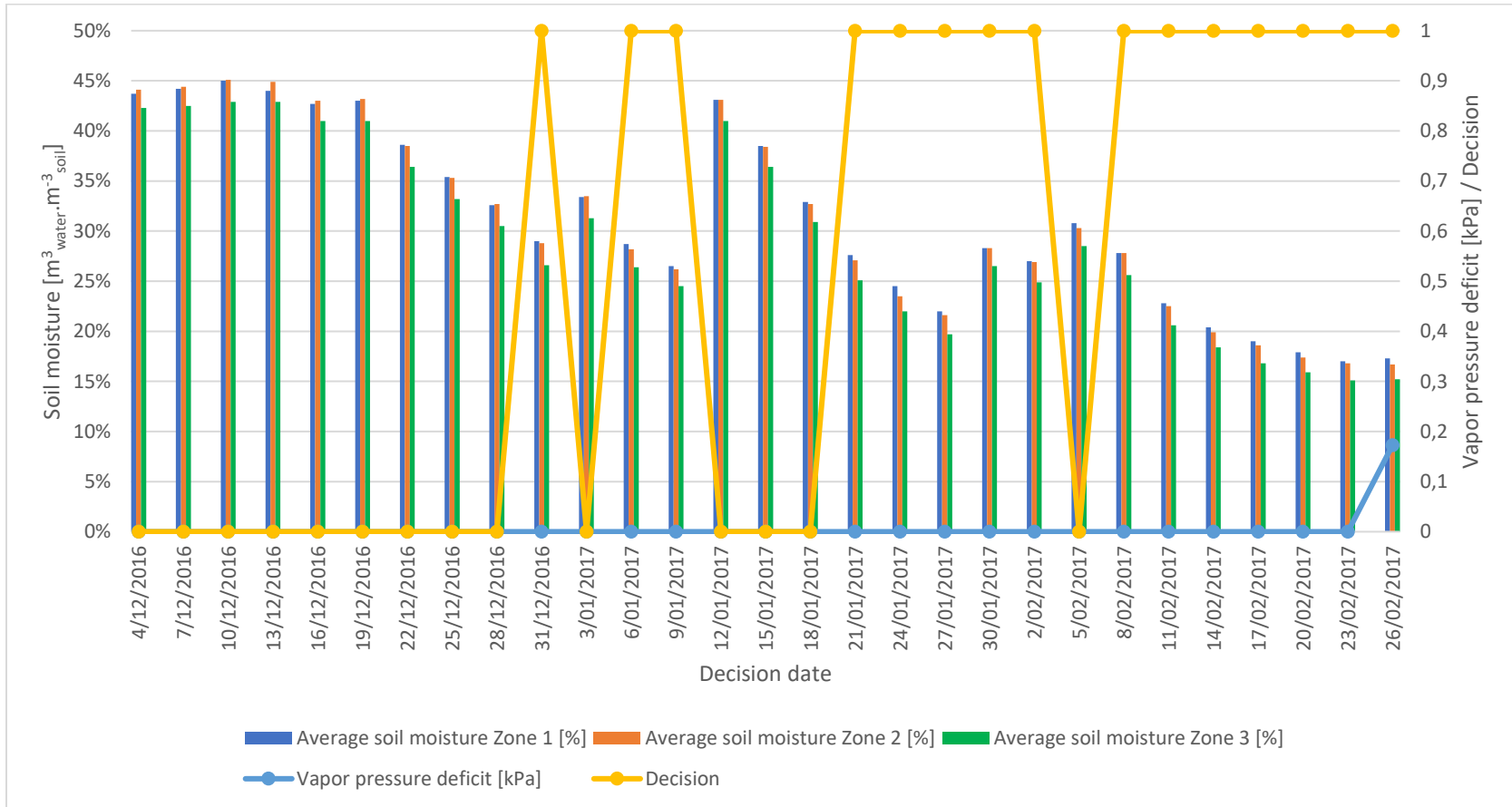
Figure 7. Irrigation decisions in relation to the average soil moisture in the 3 zones of the plot and the vapor pressure deficit for period 6.
