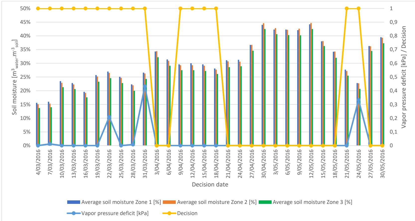
Figure 4. Irrigation decisions in relation to the average soil moisture in the 3 zones of the plot and the vapor pressure deficit for period 3.
