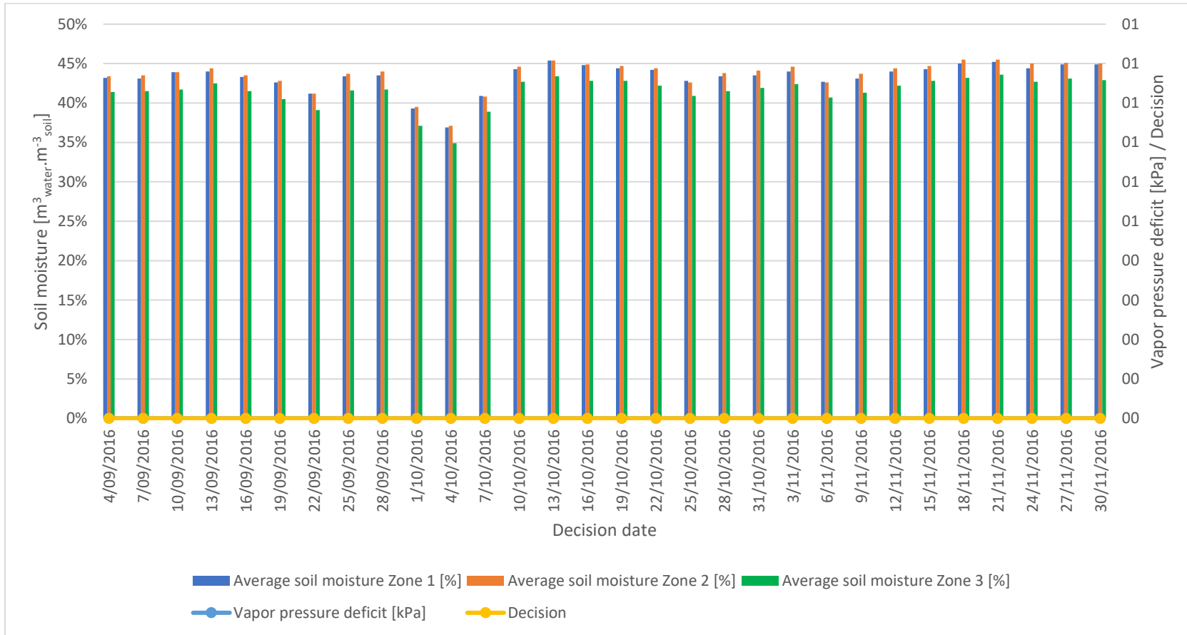
Figure 6. Irrigation decisions in relation to the average soil moisture in the 3 zones of the plot and the vapor pressure deficit for period 5.
