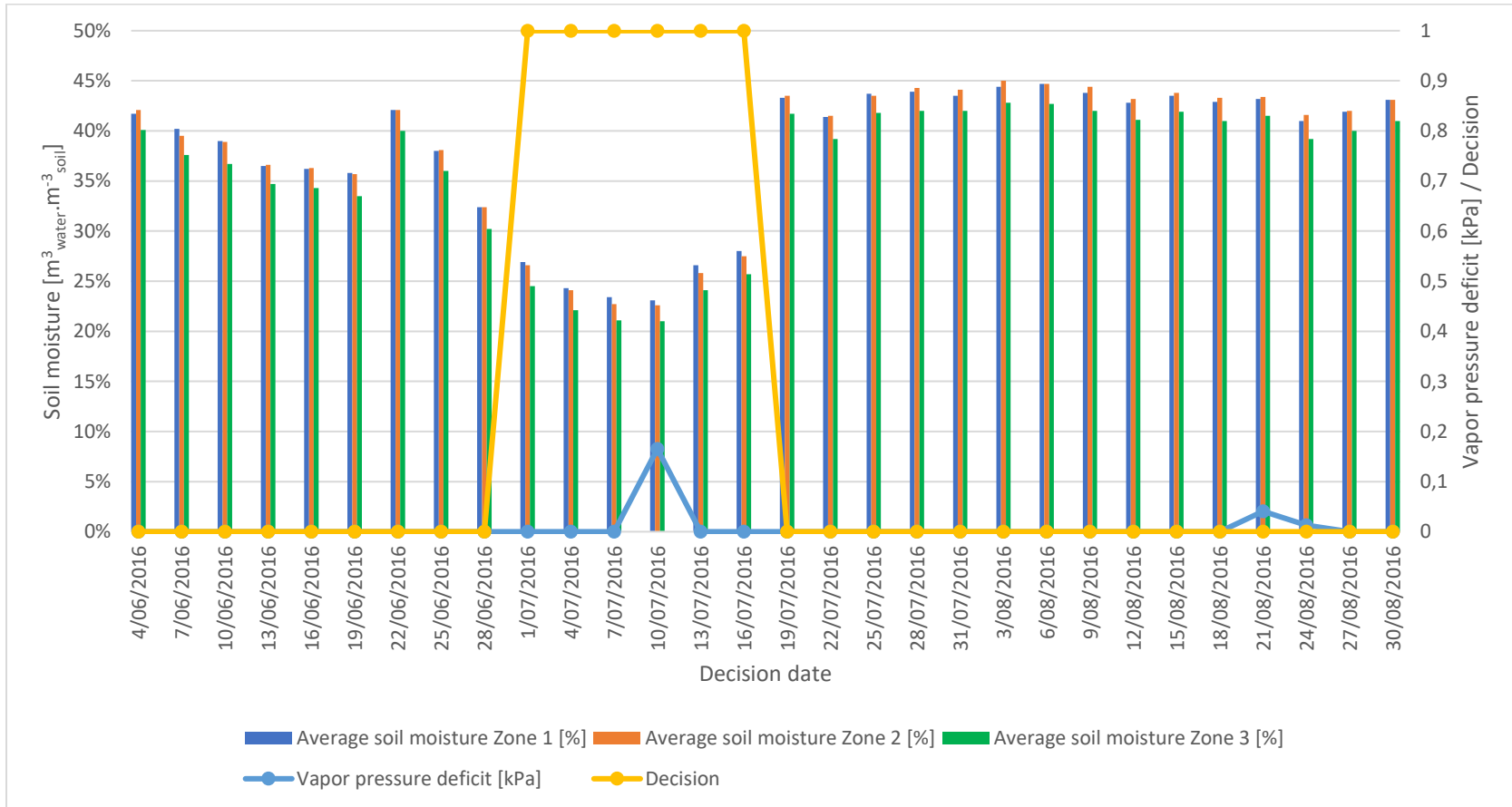
Figure 5. Irrigation decisions in relation to the average soil moisture in the 3 zones of the plot and the vapor pressure deficit for period 4.
